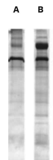
Fig 2.1. Comparison of SDS-PAGE Clean-Up Kit with ethanol precipitation. (A) Urinary protein precipitated with 10 volumes of ethanol. (B) Urinary protein precipitated with SDS-PAGE Clean-Up Kit. More and stronger bands are detected after use of SDS-PAGE Clean-Up Kit due to the efficient precipitation procedure the kit is based on. Gel: 8 × 9 cm, 12.5% acrylamide, 0.1% SDS, run on SE 260 Mini-Vertical Unit. Stain: Coomassie Blue R-250.
