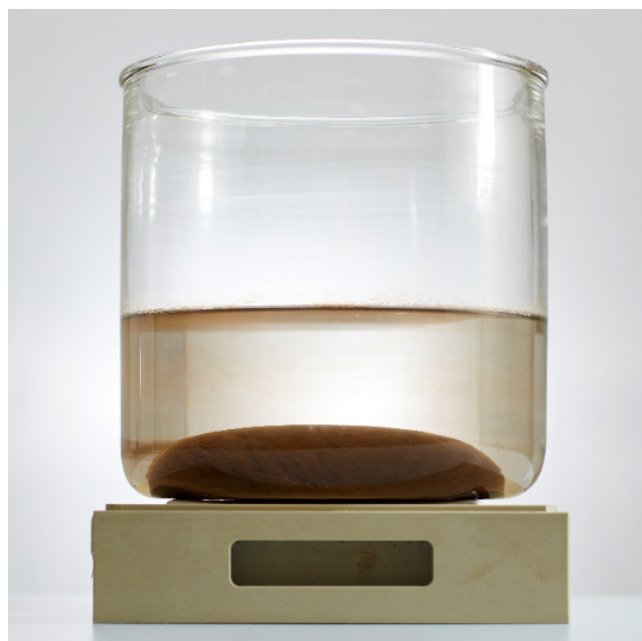
Fig 1. Example of magnetic bead separation.
