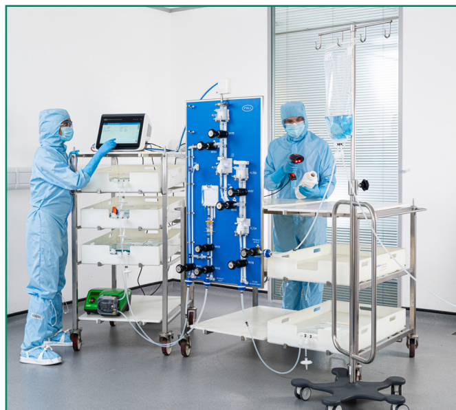
Figure 3 A shadow board concept in use with a PUPSIT capable SUS and automated filtration skid
