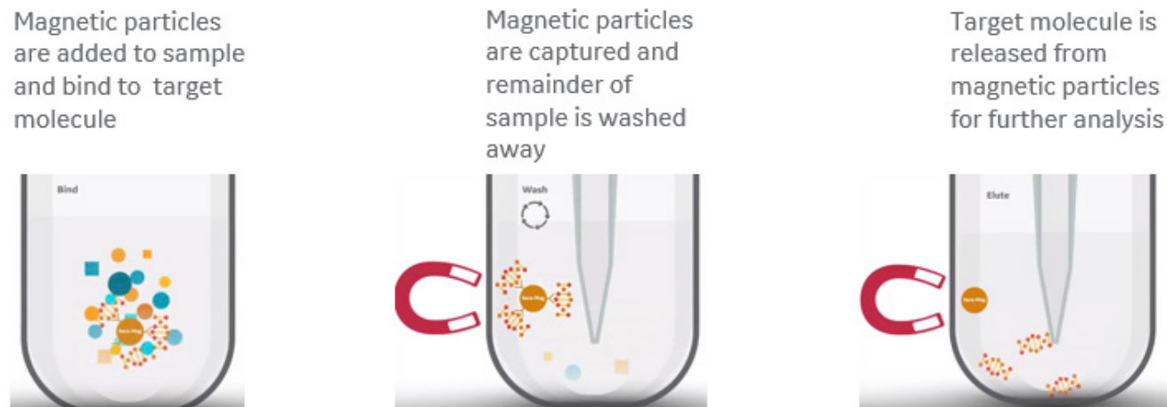
Figure 1. Overview of magnetic bead-based DNA extraction using Sera-Mag™ beads.
